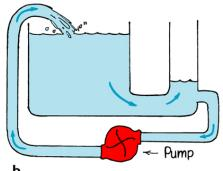
Can get sustained water flow if pressure difference maintained via a pump
