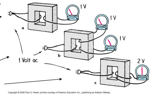
Eg. If secondary has less # turns than first, the voltage induced will be less, ie. *stepped down*.
