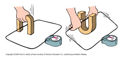
The key point is that the conductor lies in a region where the magnetic field changes
