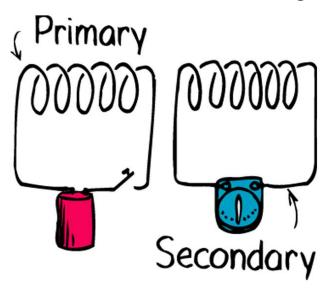
The primary coil has a battery, so when switch is closed, current flows in it, creating a sudden magnetic field that threads the secondary coil – inducing current pulse in it too. (Note no battery in secondary coil).
