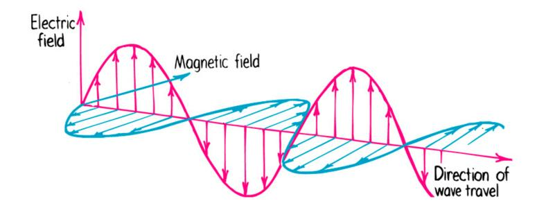
• The EM wave moves outwards (*emanates*) from the vibrating charge.
